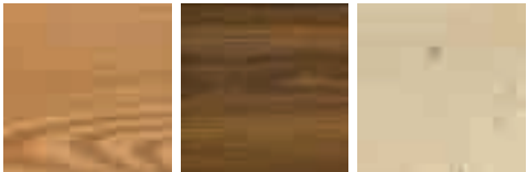
Larch Steam-treated Larch Thermo-heated 185° Spruce 12% dry
